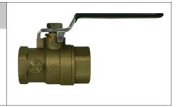
Hays Plumbing No-Lead Full Port Ball Valves with drain are constructed from heavy duty no-lead brass They are designed for residential and commercial use on steam, oil, water or gas. The full port allows for maximum flow, minimum pressure drop and turbulence. The drain feature allows for drainage of water down line to prevent freeze up.
